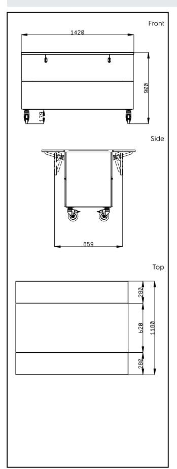
Flexy Compact Ambient unit on cupboard (4GN) with wheels, H=900mm
